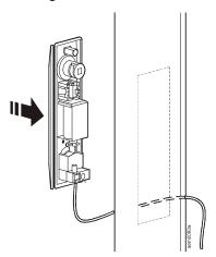
b. Place the rear cover on the handle and insert the screws to secure the handle in place. Alternate between the screws while tightening them to prevent skewing of the handle.
