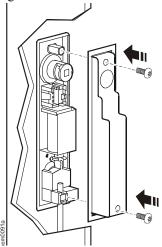
Install the cam washer and cam on the handle. For the rear handle, use the cam removed in step 1. For the GlobalFrame rack, use the removed cams for both handles.
